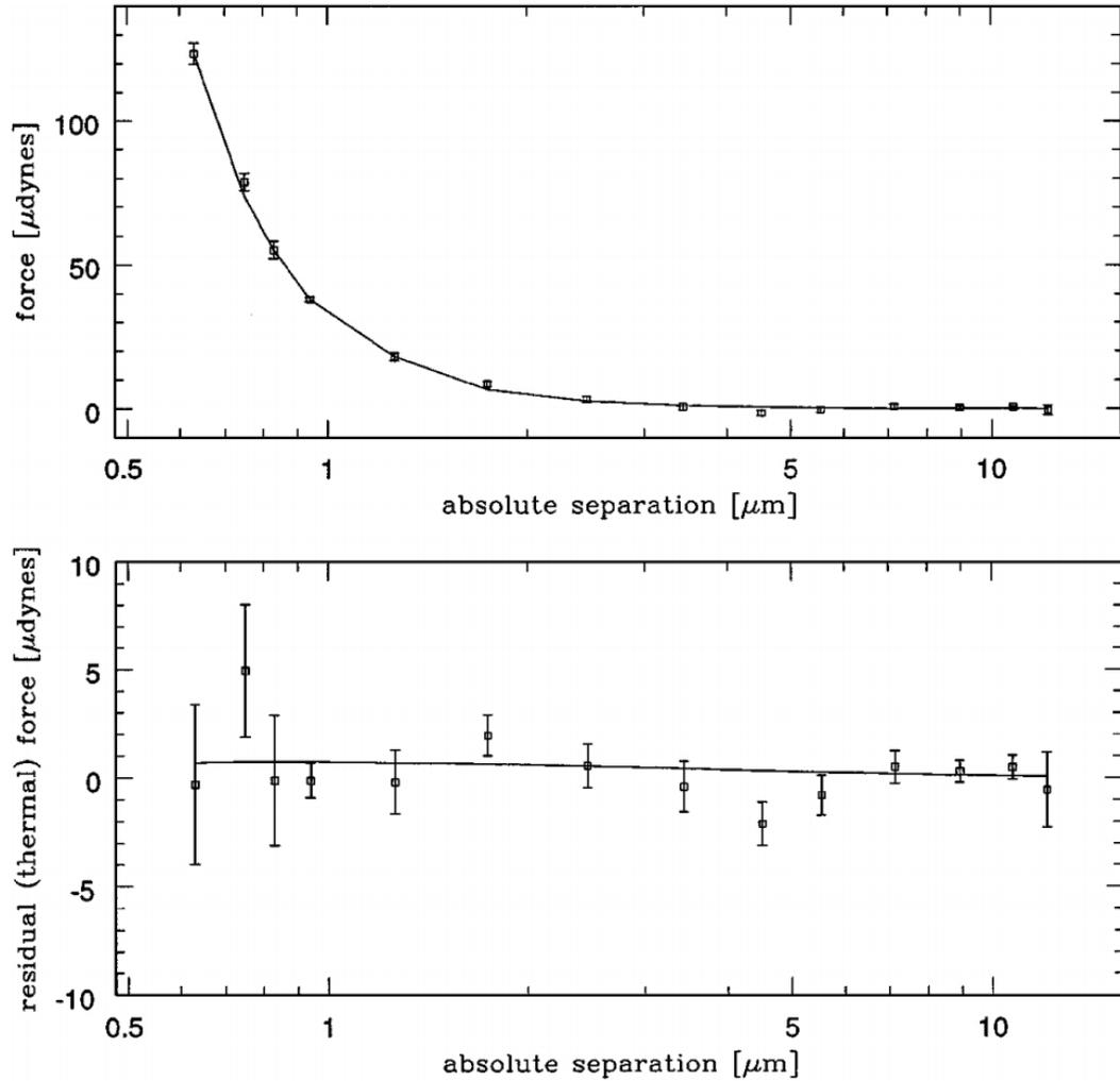
**Figure 3.2:** An experimental demonstration of the Casimir effect, measured by *Lamoreaux* in 1997. The top graph is the total force measured, the second graph is with the theoretically predicted Casimir effect subtracted off. This shows thermal residual forces. From <https://doi.org/10.1103/PhysRevLett.78.5>.
