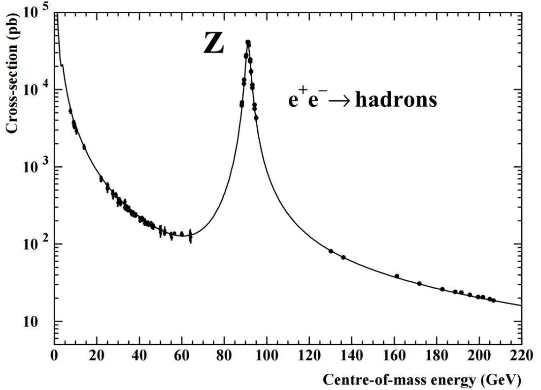
**Figure 5.1:** Cross section for an electron-positron collision to produce hadrons. The black dots are experimental results, and the solid line is the Standard Model prediction. The peak is caused by the existence of the  $Z$ -boson, which has a mass of 91 GeV. The image has been taken from *arXiv:hep-ex/0509008v3*.
